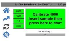
**Setup** (**(**) screen is where configuration changes can be made. In the Setup screen, you can customize the instrument according to needs and preferred operation at any time during normal operation. The Setup screen has been sub-menus split into to facilitate instrument configuration. This is also where logged files and calibration logs can be downloaded and where new software. when available. can be uploaded.
