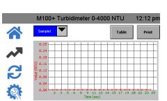
**Calibration (2)** screen is used for calibration. The instrument was calibrated and tested prior to leaving the factory. Therefore, it is possible to use the instrument directly out of the box. Under normal conditions, re-calibration is required once every three months. Quarterly calibration ensures performance within accuracy specifications.
