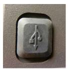
**NOTICE** A USB- Type B plug is provided at the back. This is currently not active but was supplied for a potential future update. Keep the supplied plug in place to prevent damage.
