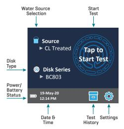
The display screen is touch-activated. To make a selection, tap the icon or word on the screen with a fingertip, fingernail, pencil eraser, or stylus.
