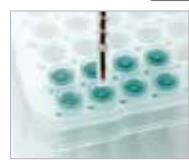
This pH electrode with temperature compensation sensor can take measurements from samples as small as 50µL, the smallest in the world.
