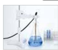
283 mm length & 8 mm diameter. The long, thin design makes this electrode perfect for measuring in large containers and test tubes.
