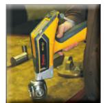
X-Ray Fluorescence Scanner provides Positive Material Identification (PMI)
