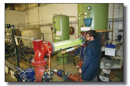
A Flow Lab equipped with a battery of water pumps is used to perform dynamic valve tests and water flow tests in a wide range of pressures and velocities to determine flow and torque characteristics of various valves. Valve test data is recorded and analyzed using a computer based data acquisition system. In addition, a 5,000 gallon air tank allows full scale air flow testing of large air valves.
