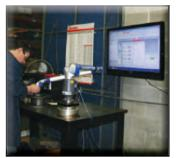
Coordinate Measuring Machine provide 3D data
