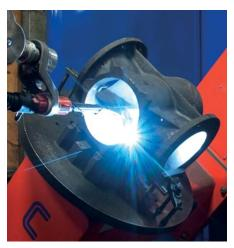
Figure 3. Robotic welding of nickel seat
